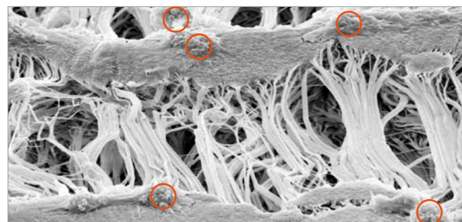
Uncoated ePTFE graft: Thrombus formation after 2 hours of blood contact 1
